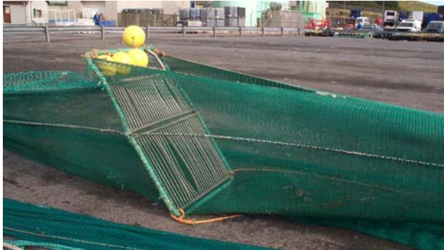
The extension of the Alison Kay 's net showing the separator grid in its operating position. The cod-end is to the left of the grid in this view and the direction of tow is towards the right. The triangular escape opening in the top of the net can be seen in front of the grid.
