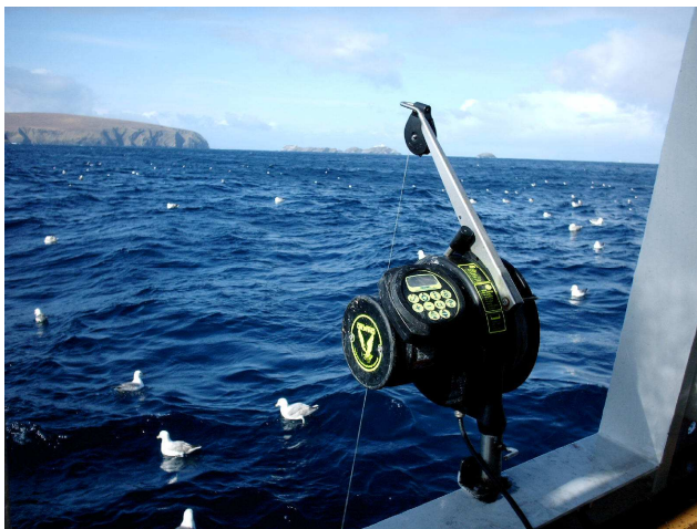
Figure 1: An Oilwind automated jigging machine installed on the NAFC Marine Centre fishing vessel Atlantia II .
